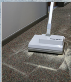
Agitate with a Dri-Way Jr. machine using a back and forth and crosswise motion working the compound into the carpet nap.
